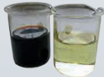
↑ Colour removal from caustic from regeneration processes
